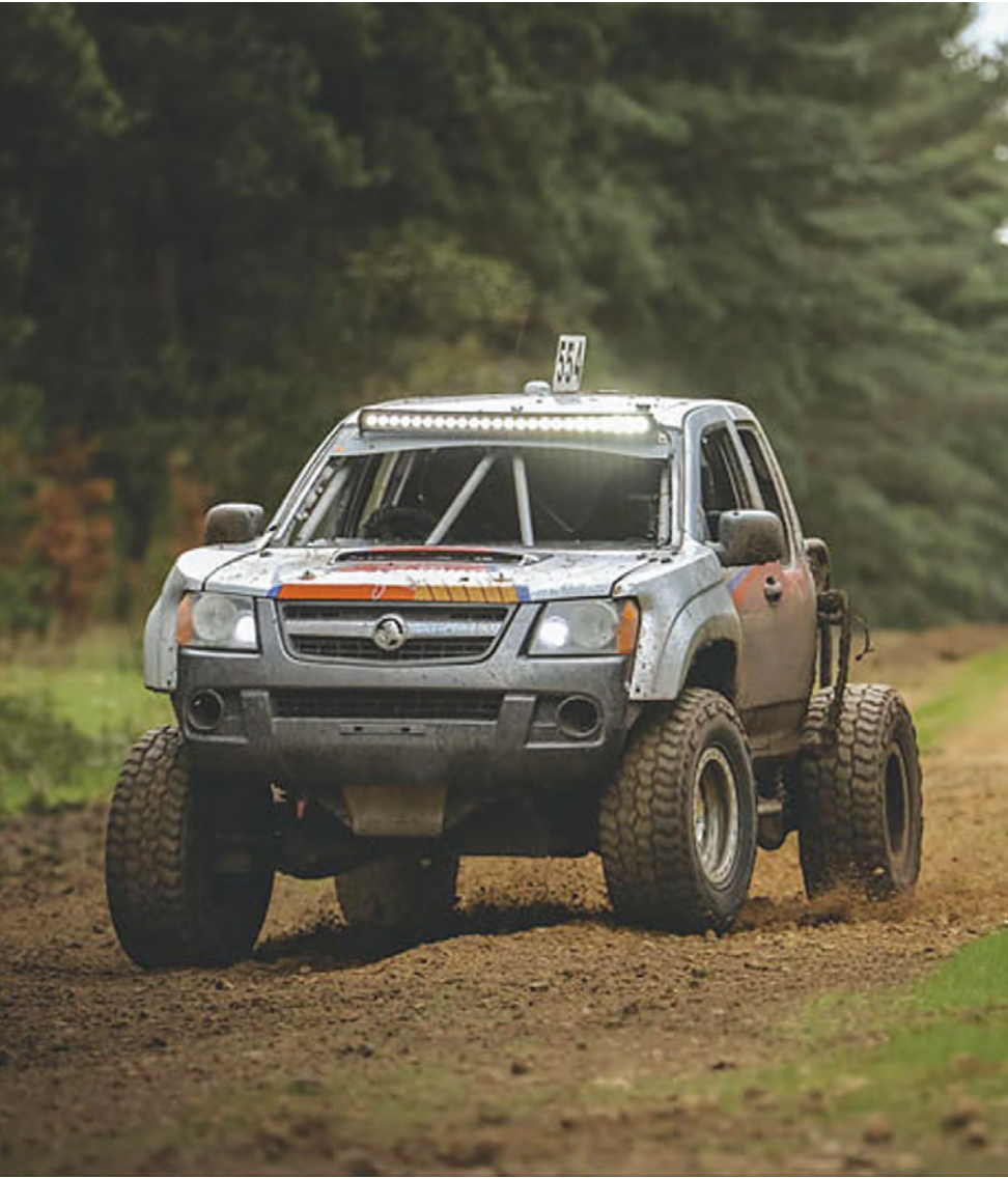
The Holden Colorado started life as a 3-litre turbo diesel 4x4, supplied by River Murray Auto Wreckers. The Dutch Courage team retained the chassis and the cab, but cut away everything else, and replaced the engine with the 6-litre V8 Holden turbo 400 trans, with a 10-inch Ford diff. Barry Sullivan custom built the suspension arms and rollover protection. The 17-inch race wheels are wrapped in Mickey Thompson Baja ATZ tyres. The car has a top speed of around 188km/h.
