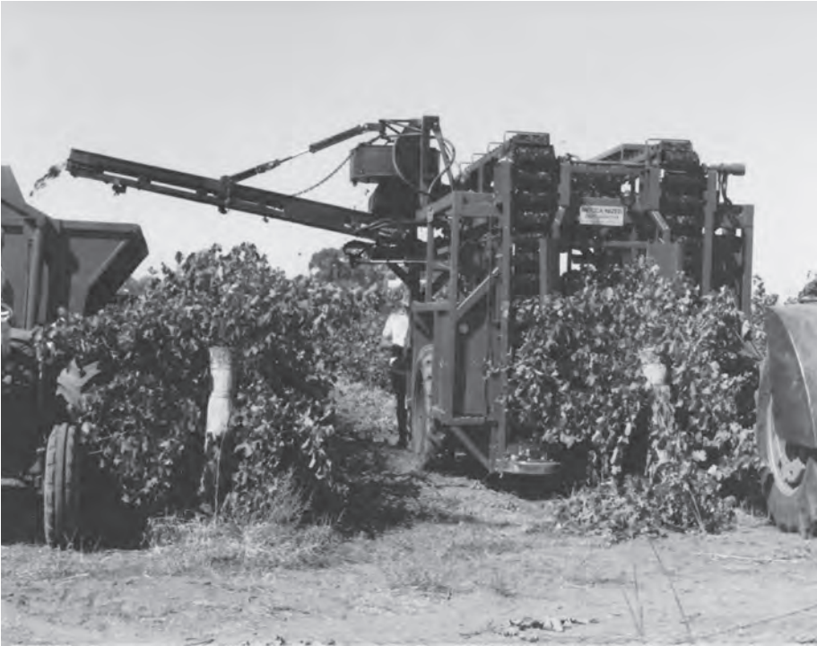
Early tractor-drawn machine harvester with accompanying tote bin, Luther Road, Loxton, 1975: During the current Riverland wine-grape season, our region is harvesting the largest portion of the nation’s wine-grapes, amounting to more than 20 per cent of Australia’s grapes and some 60 per cent of South Australia’s total. The days of handpicking are long superseded. In an innovative global first, from the late-1960s the now rather finely-tuned machine harvesters were first developed for commercial production by – among others – CSIRO Merbein, Victoria, scientists Dr Peter May and Peter Clingeffer in collaboration with USA colleagues including Dr Nelson Shaulis, Cornell University. For the machines to work effectively, the vines needed to be retrained on specifically designed trellis systems. This development corresponded with the growing of grapes on vine rootstocks, native to eastern-USA and resistant to pests like phylloxera and nematodes and to soil factors like lime or drought. This required a significant change in vineyard production systems but allowed the new harvesters to pick up to 200 tonnes of fruit in the cool of night in air-conditioned comfort, whereas good hand pickers could harvest about one tonne a day, enduring both the heat of late-summer afternoons or the cold of frosty autumn mornings. PHOTO: Gary Luitjes
