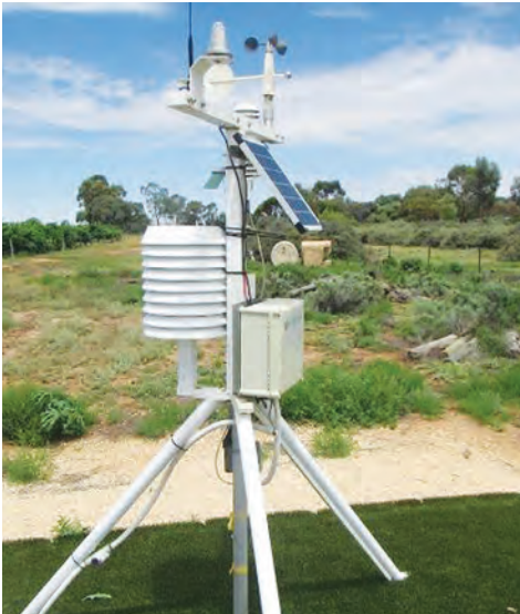
One of the MRLB's automatic weather stations. PHOTOS: supplied
