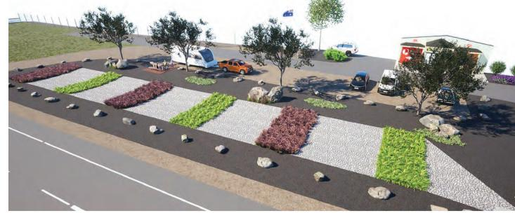
Conceptual designs for the shallow rock swale and beatification to be undertaken at the intersection of Anderson Terrace and Turnbull Terrace in Glossop as part of council's stormwater management. IMAGE: Berri Barmera Council
