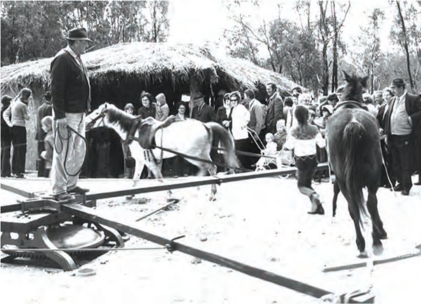
Horse-works being demonstrated at the Loxton Historical Village, September 1973: This device consisted of a horizontal, domed, gearwheel about 1 metre in diameter, and brackets for four poles upon which the man is standing. The poles connected to a harness on the horses so that as they walked the circle around the machine, the horizontal gearwheel was turned. This wheel meshed with a small, bevelled gearwheel, which turned a shaft connected to implements in the thatch-roofed chaff shed. Horses had long been used to pull wagons for transport and ploughs for tilling the soil but, in Australia, horse-works came into use in the 1840s. Before this, farmwomen and children often operated chaffcutters, grinding machines or winnowers by hand. The horse-works were gradually replaced when engines powered by oil, petrol, or kerosene came into use from the early-1900s. Horse-works of a similar design, but known as horse-whims, were used to lift diggings from mine shafts, and others known as horse-mills, linked directly to millstones to grind wheat and other cereals. Out in the paddock, some farmers used a sloping, moving belt as a treadmill upon which the work horse walked to power farm implements such as winnowers and chaffcutters. PHOTO: LHV
