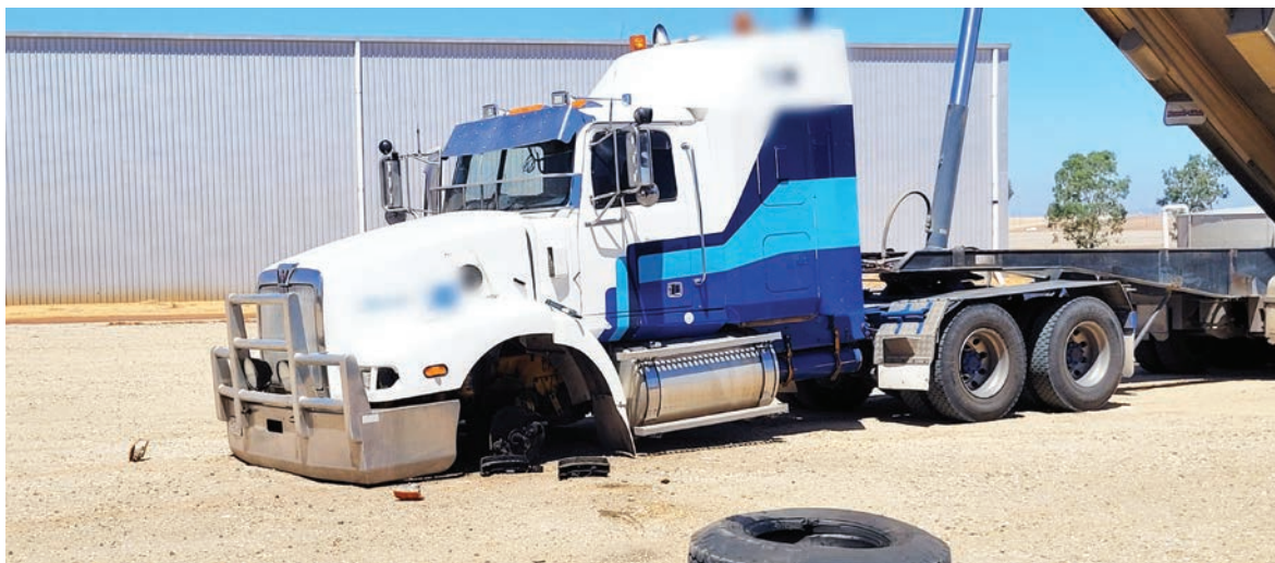
SA Power Networks is urging farm safety after this truck's wheels were blown off when the tipper contacted an 11,000-volt powerline. Fortunately, the driver was uninjured. PHOTO: supplied
